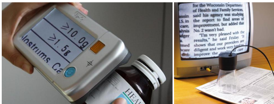
Figure 14. a) A Digital Portable Magnifier, b) A Video Reading Magnifier. (Source: http://www.thebrailledpot.com/Low_Vision/Eye_Q.html and http://www.maculardegeneration-reader.com/eazyreader )
