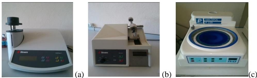
Figure 3.7. Devices used in the experiments (a) Hot mounting press (b) Low speed diamond saw used for cutting samples (c) Polishing machine
