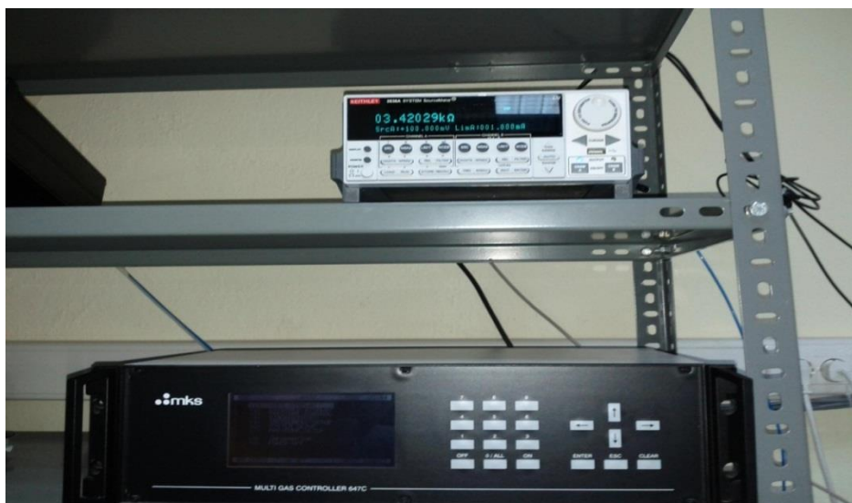
Figure 3.5. MKS 647C and Keithley 2636A Sourcemeter
