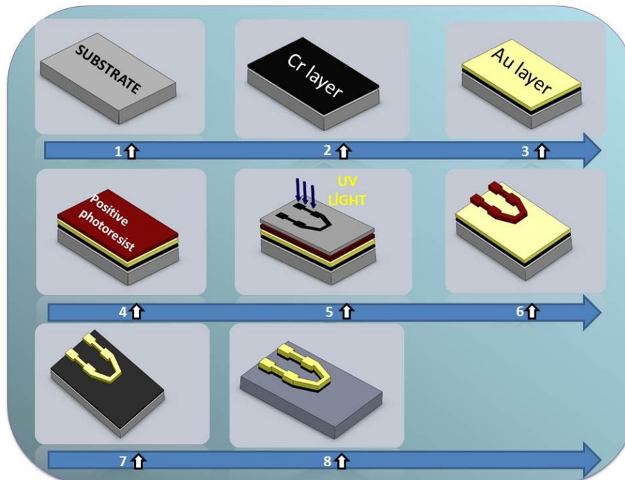
Figure 3.10. Photolithography steps. (1) cleaning, (2) Cr film deposition, (3) Au film deposition, (4) positive resist coating, (5) UV light exposure, (6) development, (7) Au etching, (8) Cr etching
