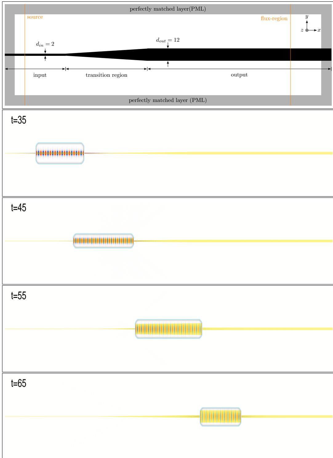
Figure 4.9. Dielectric profile of waveguide consist of input region with thickness of  $d_{in} = 2$ , trapezoidal taper region and output region with thickness of  $d_{out} = 12$ . All waveguide region have same dielectric constant of  $\epsilon_a = 13$ . The waveguide structure immersed in a background with dielectric constant of  $\epsilon_b = 2.25$ . Electric field profile of TE mode taken at four different time along waveguide that is adiabatically connected with a transition region.
