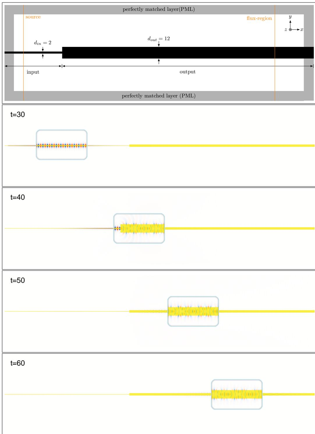
Figure 4.8. Dielectric profile of waveguide structure consisting of two butt joined single-slab. Input slab has thickness of  $d_{in} = 2$  with dielectric constant of  $\epsilon_a = 13$ . Output slab has thickness of  $d_{out} = 12$  with dielectric constant of  $\epsilon_a = 13$ . FDTD simulation of electric field distribution of waveguide structure that is made by butt joined single-slabs.
