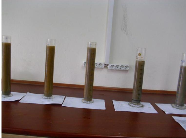
Figure 3.2. Hydrometer Tests Performed in this study
