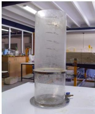
Figure 5.11. 1-D Test Equipment
