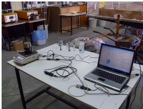
Figure 6.5. A Hyprop Test is in Progress
