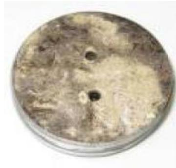
Figure 4.7. Soil Sample with Two Shaft Holes
