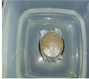
Figure 6.1. Dish with Water and Sample during The Initial Saturation Process.
