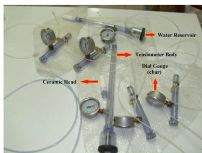
Figure 5.14. Parts of the used Tensiometers (Model:T5-2100F)
