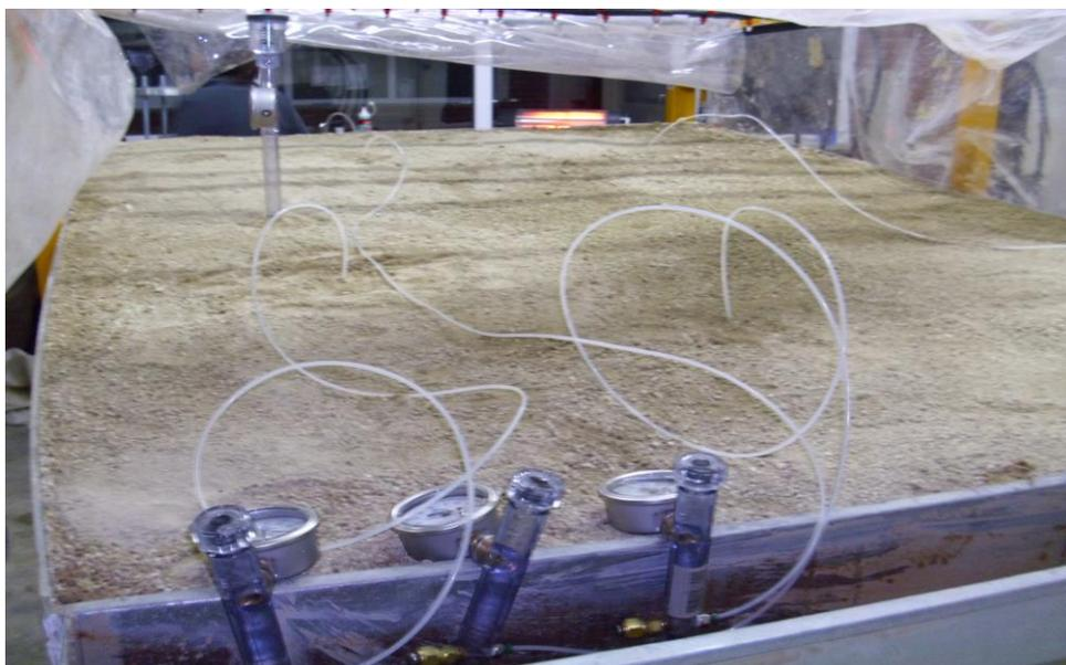
Figure 5.7. Another View of The Filled Soil Container and Placed-in Tensiometers
