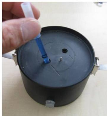
Figure 4.6. Assembly of the Tensiometer
