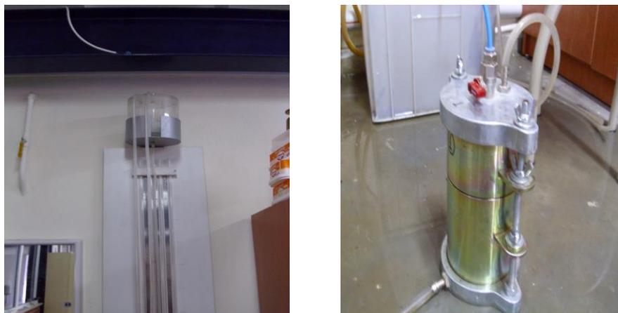
Figure 3.23. Falling Head and Constant Head Permeability Test-Equipment
