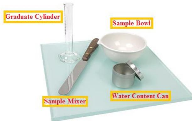
Figure 3.7. The Plastic Limit (PL) Test Equipment
