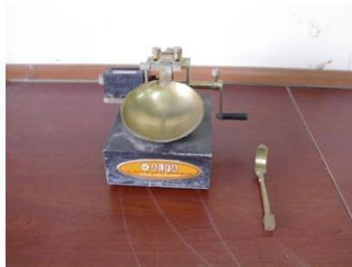
Figure 3.5. Casagrande Apparatus used for the Multi-Point Liquid Limit Test
