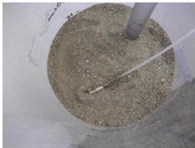
Figure 5.13. To Assembly a Tensiometer in 1-D Test Set-Up
