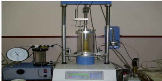
Figure 3.21. Automatic (Static) Triaxial CU-Test set-up used by (Ege University Geotechnical laboratory) (Source: Pulat, H.F, 2009)
