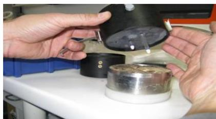
Figure 6.2. Assembling the Hyprop's Sensor Unit with the Sampler Ring
