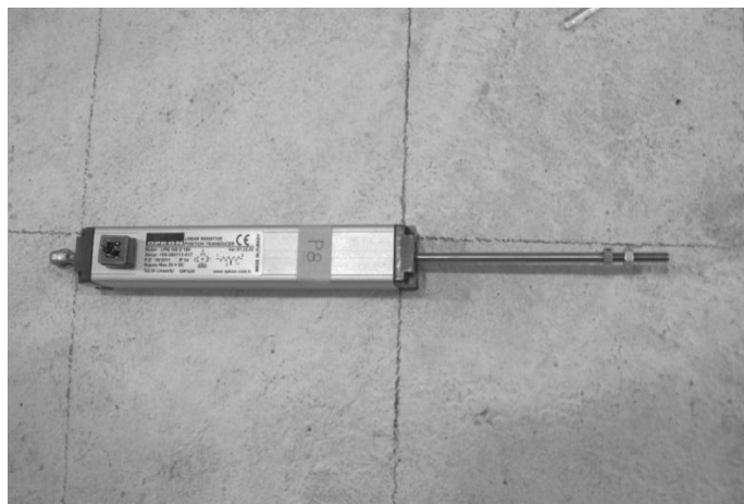
Figure 3.9. Resistive Linear Position Transducer
