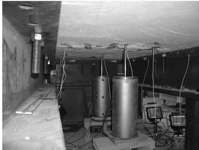
Figure 2.2. Sensor locations and support conditions (Source: Zinnedin, 2007)
