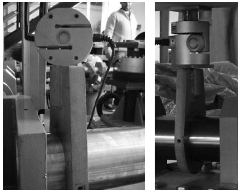
Figure 3.17. 5000 kg (on the left) and 10000 kg capacity (on the right) load cells on the hinge
