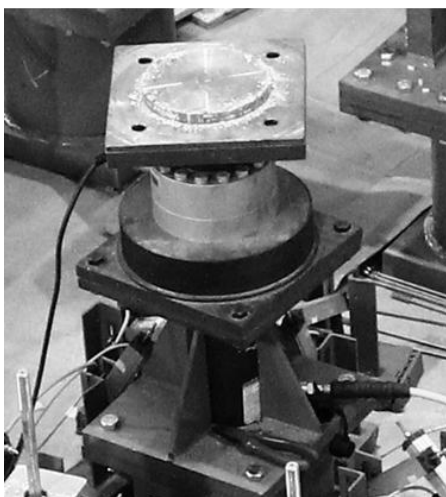
Figure 3.7. Hydraulic jack with the load cell
