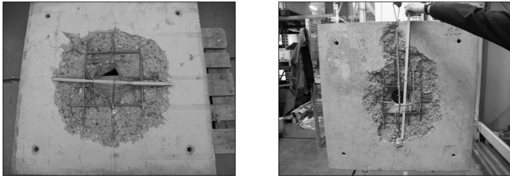
Figure 2.13. Slabs with standard steel reinforcement (B3, left) and additional stirrup reinforcement (B4, right) (Source: Hummeltenberg et al., 2011)
