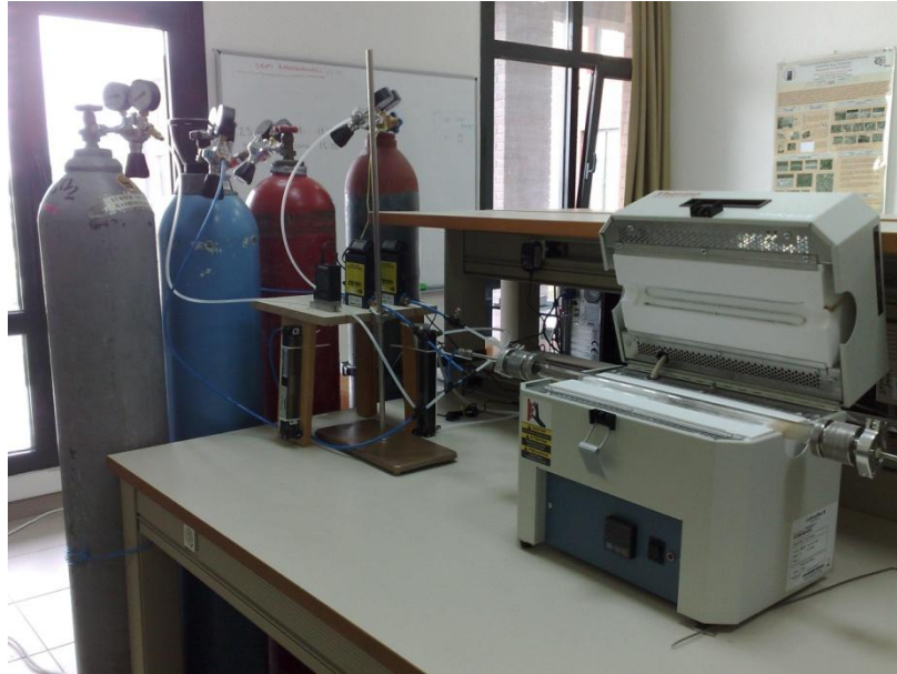
Figure 4.2. The TCVD System at CNL Lab at Physics Department, IYTE
