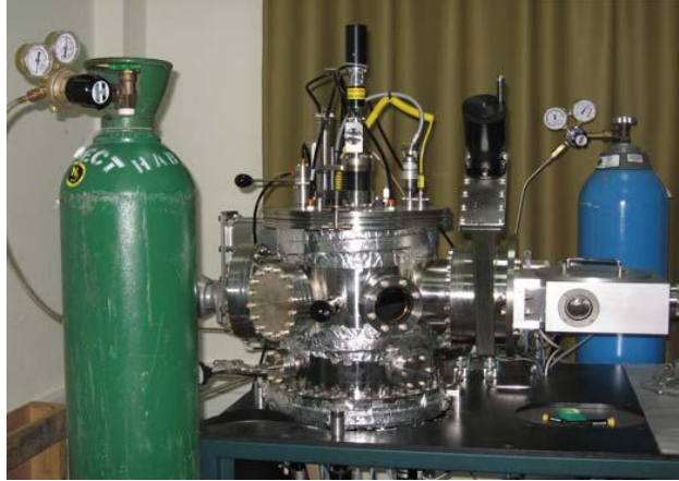
Figure 4.1. The Magnetron Sputtering System in Physics Department, IYTE
