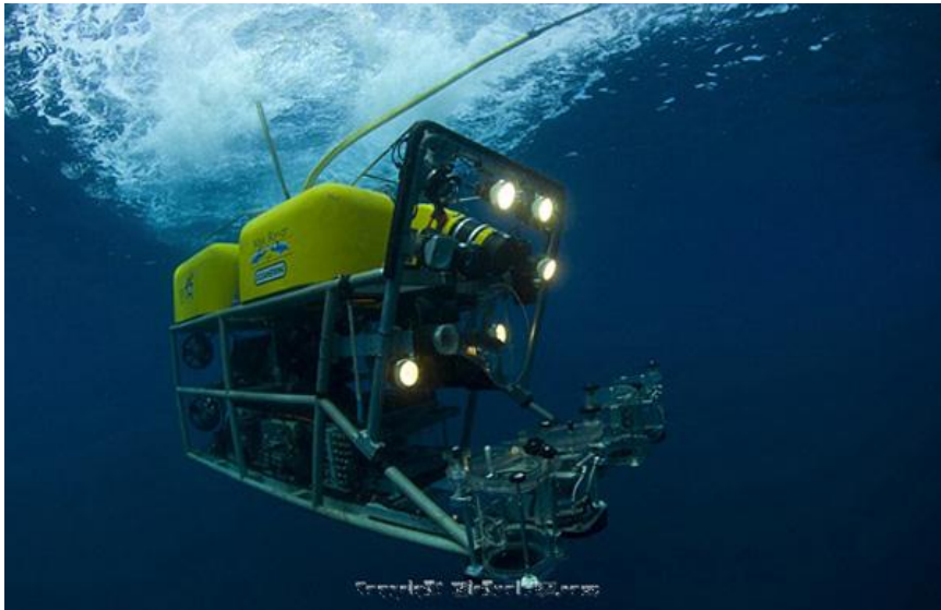
Figure 1.5. Remotely operated vehicle for underwater operations. (Source: Oceanexplorer 2012)
