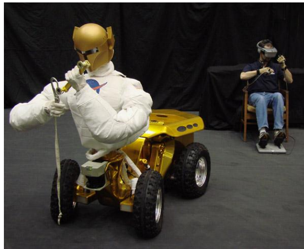
Figure 2.5. Robonaut teleoperated robot developed in NASA with telepresence. (Source:Robonaut 2012)
