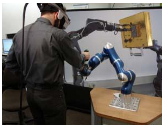
Figure 2.4. Visual telepresence with goggles. (Source: Dlr 2012)
