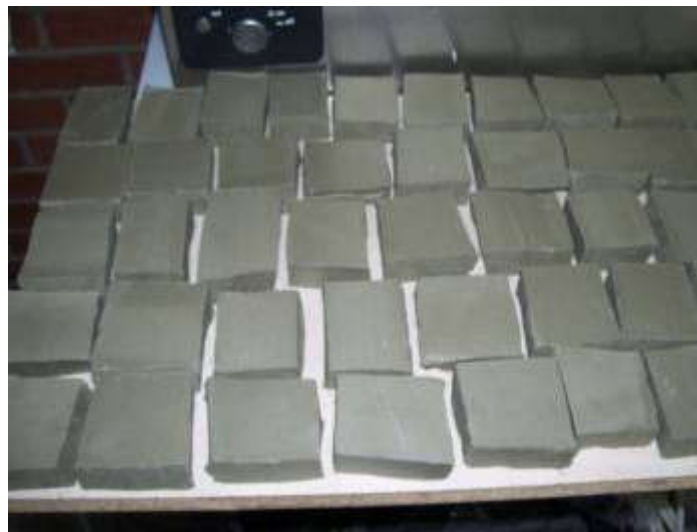
Figure 3.2. Green roof tile samples that were wire-cut.
