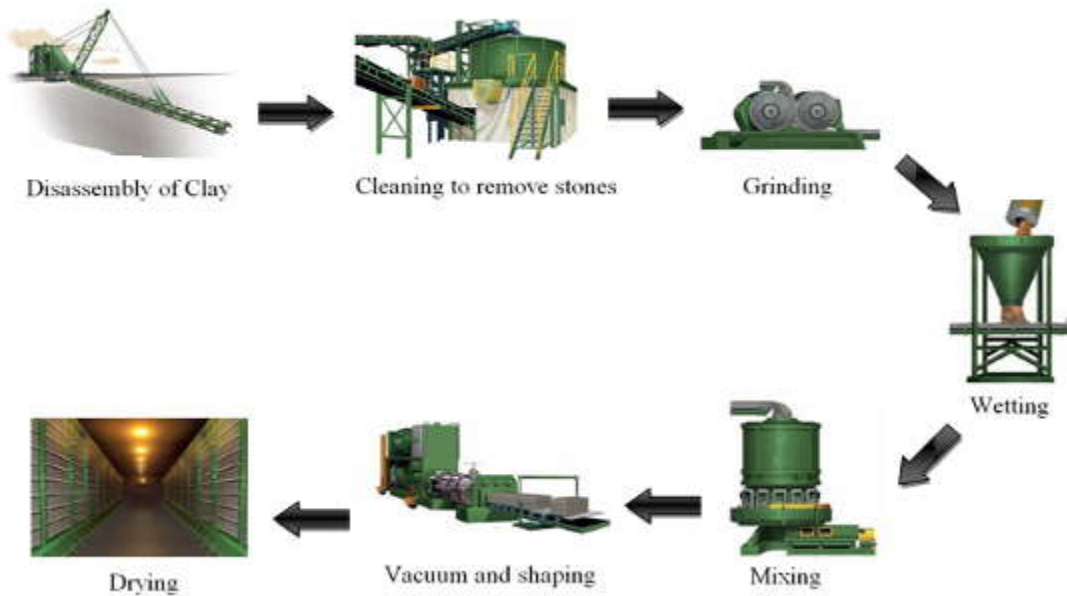
Figure 3.1. Manufacturing of roof tiles (Source: Wienerberger 2009).
