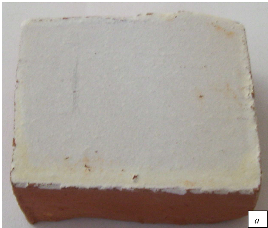
Figure 4.25. Image of the HP engobe samples prepared with 20%w lab frit. These results are to be compared to Figure 3.10. a)EHP1-20, b) EHP2-20 and c) EHP3-20
