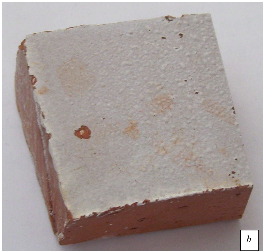
Figure 4.48. Image of the LP engobe samples ground at different speeds a) ELP-IF-12-200, b) ELP-IF-32-200.
