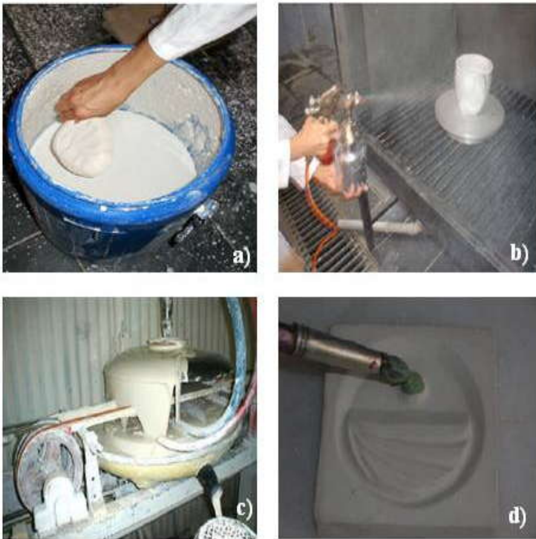
Figure 2.8. Application methods of the engobe: a) dipping b) spraying c) waterfall and d) brushing (Source: MEGEP 2007).
