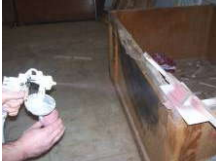
Figure 3.7. Application of engobe with a spray gun.
