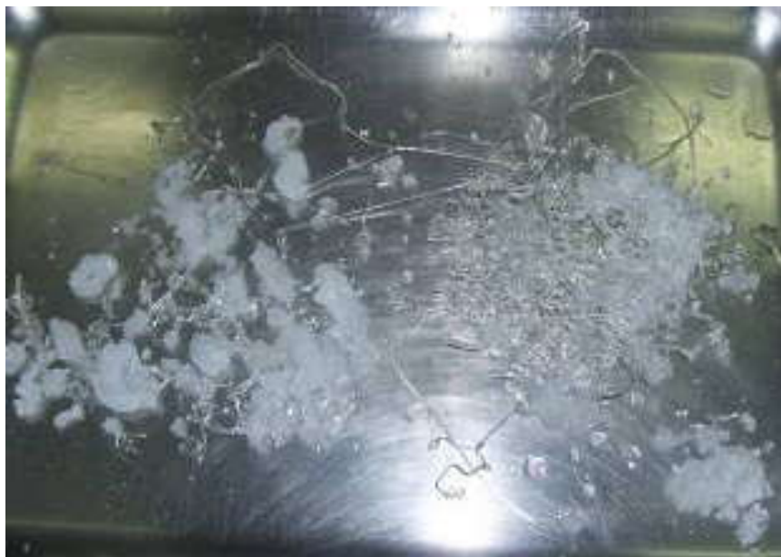
Figure 4.21. The Laboratory Frit (18% B_2O_3 ) removed from water was glassy.
