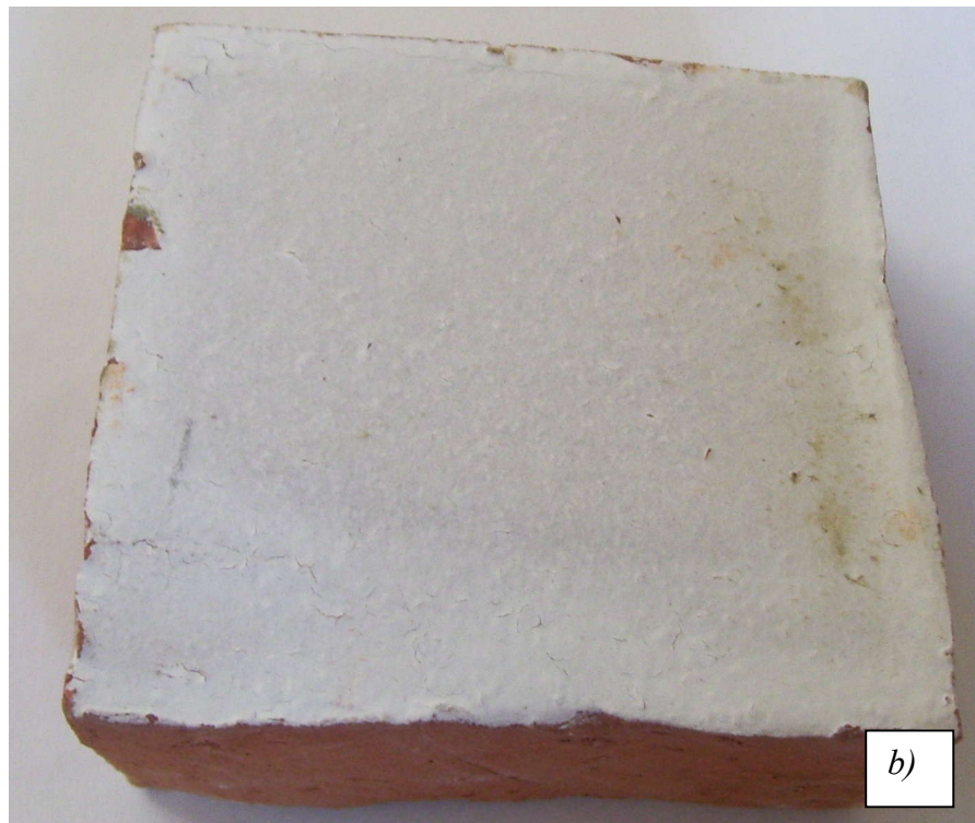
Figure 4.26. Image of the HP engobe samples prepared with 30%w lab frit. These results are to be compared to Figure 3.11. a)EHP1-30, b) EHP2-30, c) EHP3-30
