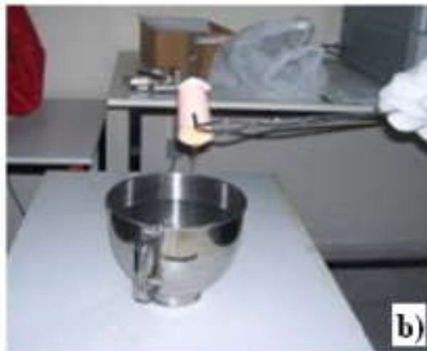
Figure 3.4. Making of frit a) melting in box kiln and b) quenching in water.
