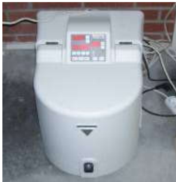
Figure 3.5. Fritsch Pulverisette 6 planetary ball mill for dry grinding.
