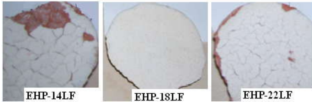
Figure 4.23. Photograph of the engobe samples with different kinds of lab frit.
