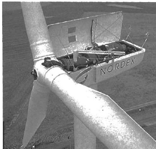
Figure 2.2. Typical nacelle cover. Reproduced by permission of Nordex AG [3]
