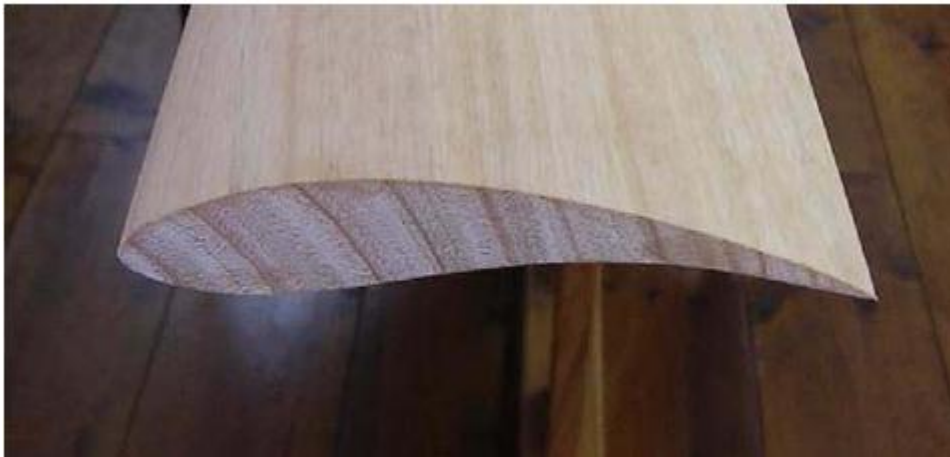
Figure 4.4. The wind tunnel model of the T.Urban 10/193 blade section [10]
