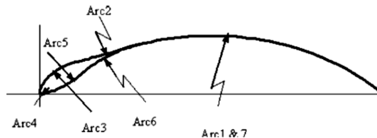
Figure 4.5.The wind tunnel model of the T.Urban 10/193 blade section [13]
