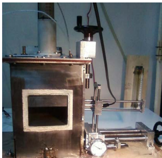
Figure 3.3. General view of test section and traverse mechanism
