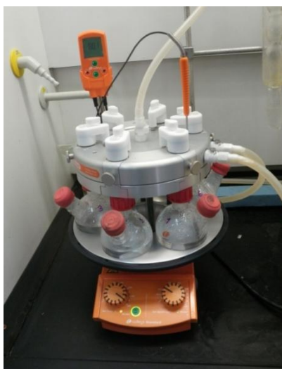
Figure 3.2. Experimental set up of synthesis of Gd doped CdTe nanocrystals
