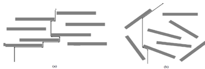
Figure 3.9. a) Regular oriented b) Random oriented silicate layers in polymer matrix (Source : Cornwelle 2009)
