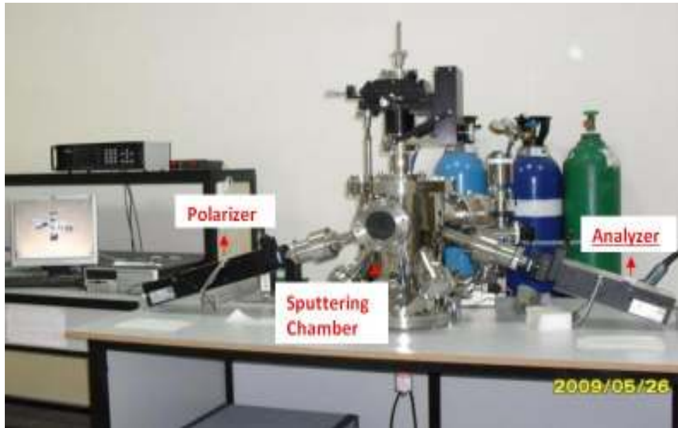
Figure 5.5. Picture of the magnetron sputtering system with SE.
