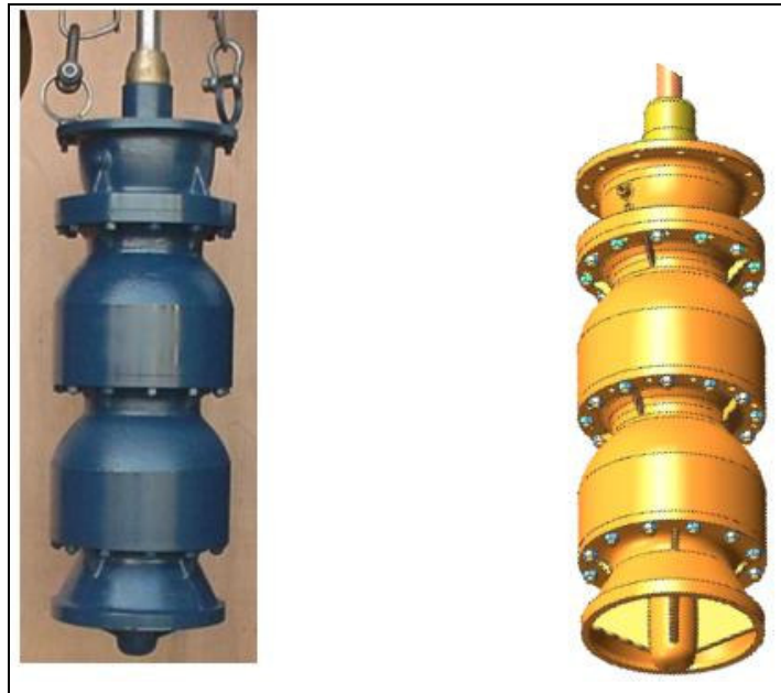
Figure 4.1. VDP 1433 with two stages and its CAD model.
