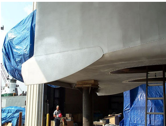
Figure 3.16. Water jet side seen (Source: WEB_2 2004)
