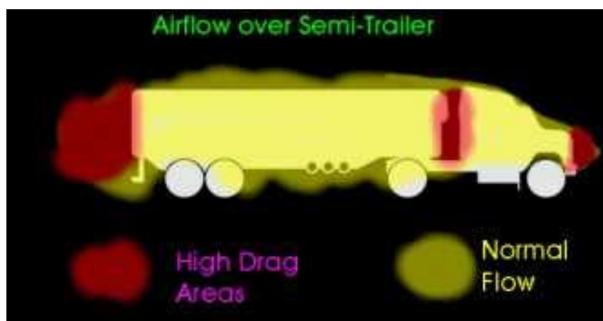
Figure 1.1. Sources of drag for a semi-trailer (Source: Web_1,2005)
