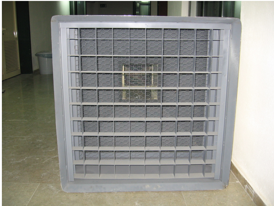
Figure 5.9. Flow straighteners inside the settling chamber
