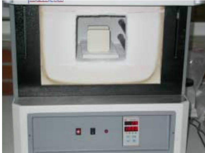
Figure 4.3. Protherm PLF 160/5- High Temperature Furnace (Max. Temp.=1600°C).
