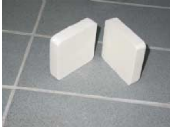
Figure 5.24. Photograph of dry pressed alumina tile sintered at 1550°C (70x70x20 mm).
