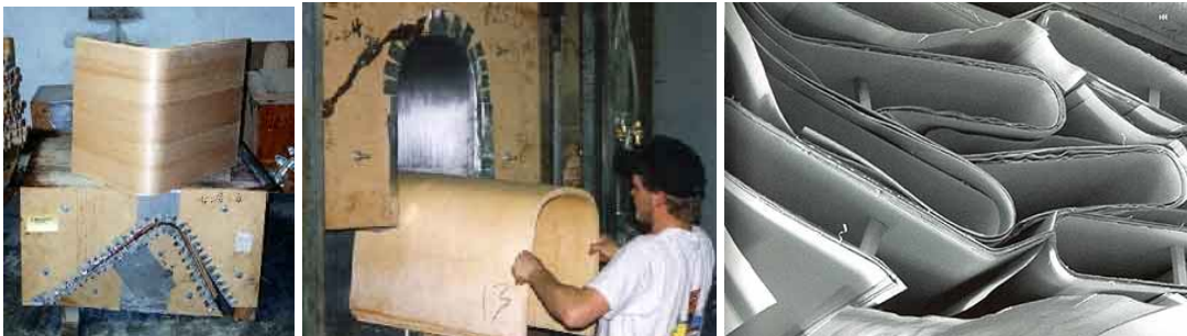
Figure 3.40: Plywood bending process, ( http://www.ahwoddworks.com/bentwoodprocess.htm )
