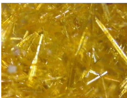
Figure 4.2 Yellow crystals of \text{PbVO}_3\text{Cl} (Nikon Eclips L150 Optic Microscope, 10 X magnitudes).
