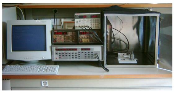
Figure 2.2 Simultaneous Capacitance-Voltage (C-V) Setup
