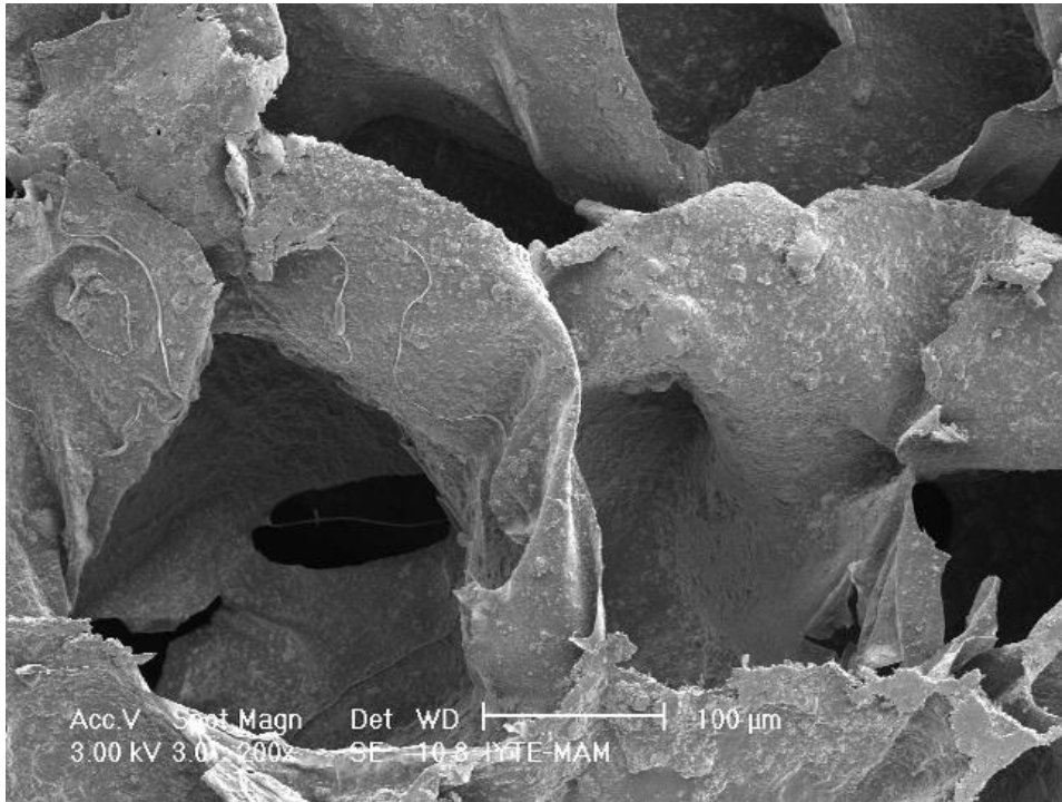
Figure5.21e) SEM of porous HA/chitosan composite, CH50, 50wt%HA.
