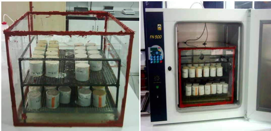
Figure 3.5. Storage system of mortar samples
