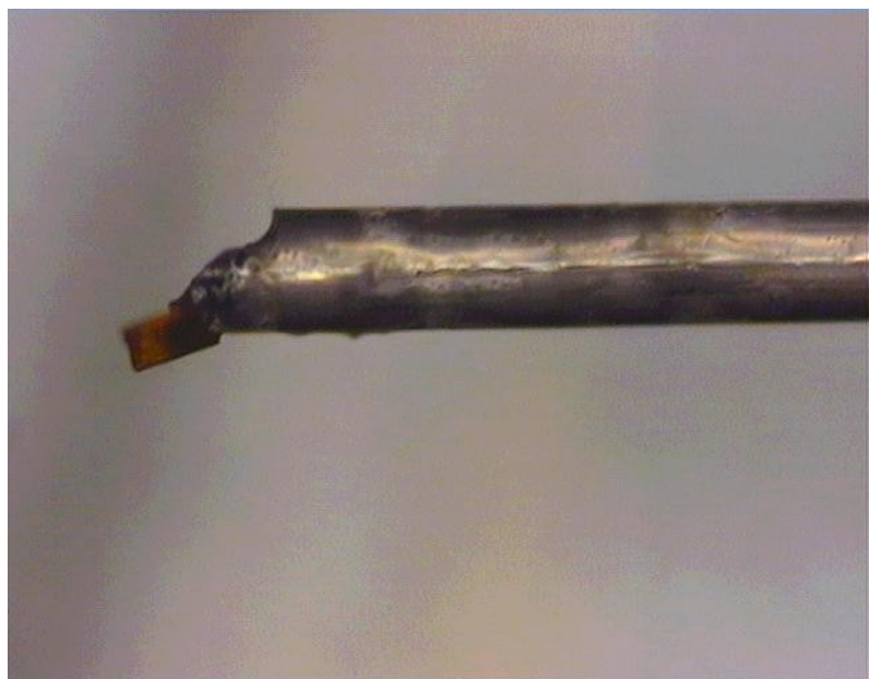
Figure 2.4 A mounted single crystal to a capillary with epoxy
