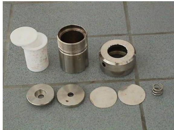
(b) PTFE cup with cover , acid digestion bomb body, screw cap, pressure plate (upper), pressure plate (lower), corrosion and rupture discs, spring.[from left to right]
