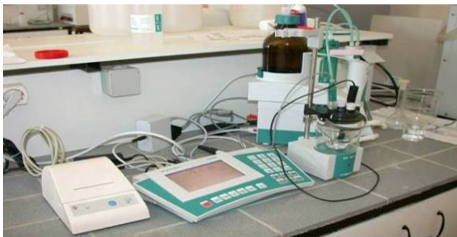
Figure 5.1. 781/pH-Ionmeter, 776 Dosimat Unit and Ammonia Selective Electrode.
