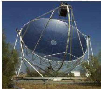
Figure 1.3. Paraboloidal dish, Eurodish
