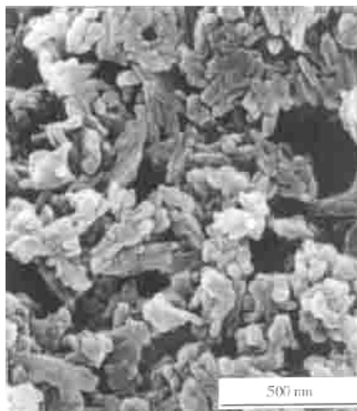
Figure 7. SEM micrograph of the as synthesized HA powder (Ca/P=1,667) (13)
