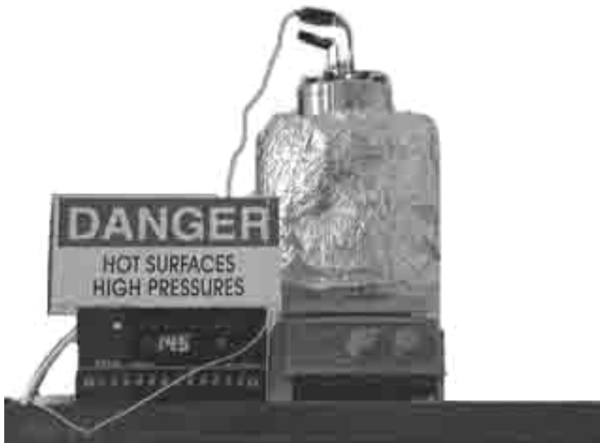
Figure 19. Photograph of the experimental setup used for the hydrothermal synthesis of whiskers.
