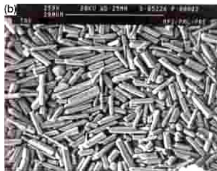
Figure 13. SEM micrograph of HA whiskers prepared by MSS (32).
