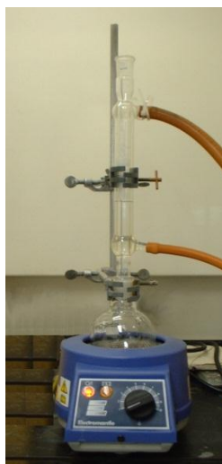
Figure 3.5. The Scheme of the Reflux System
