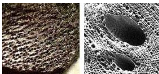
Figure 4.7. Structure of active carbon (SEM visualization)
