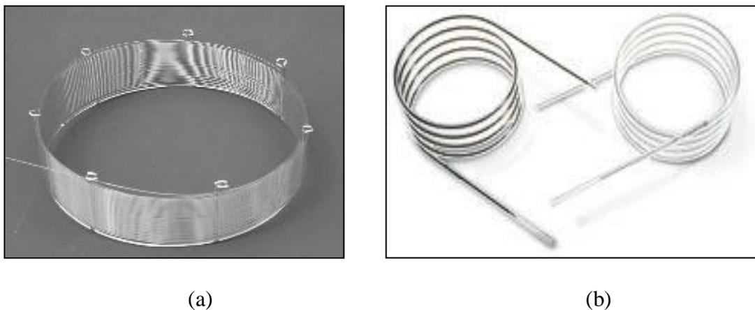
Figure 2.2. Column types (a) Capillary columns, (b) Packed columns
