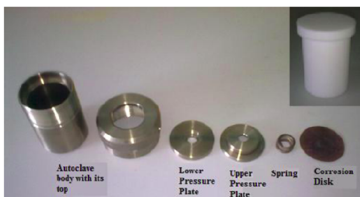
Figure 2.2. Schematic representation of an autoclave with its parts.
