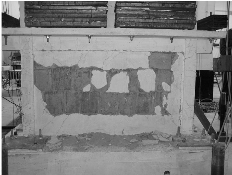
Figure 3.25. Damage of the first story at the end of the sixth loading group south face
