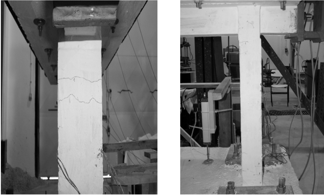
Figure 3.13. Flexural cracks at the east face (left) and shear crack initiation at the south face (right) of the first story east column, at the end of the first loading group
