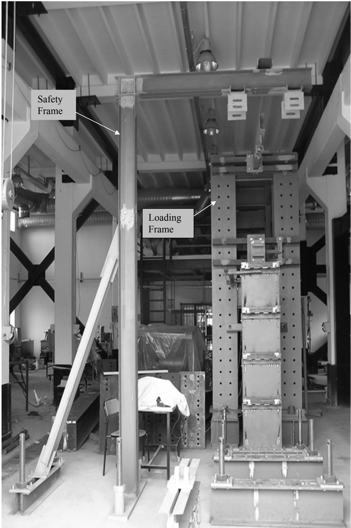
Figure 2.14. Loading and Safety frames
