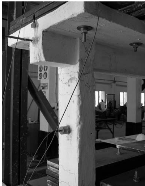
Figure 2.18. Typical attachment of accelerometers on mid height of the columns and slabs
