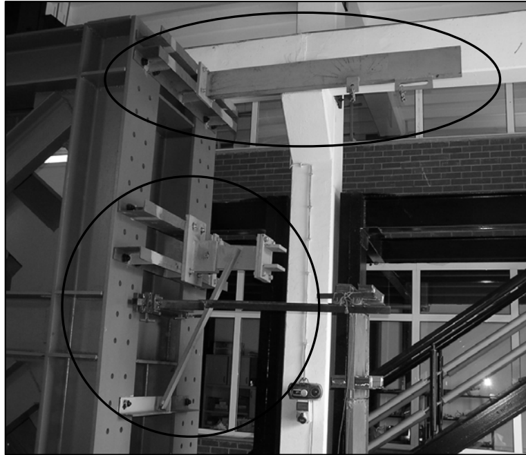
Figure 2.12. In-plane hanging frame (top) and hydraulic cylinder attachment at loading system (bottom)
