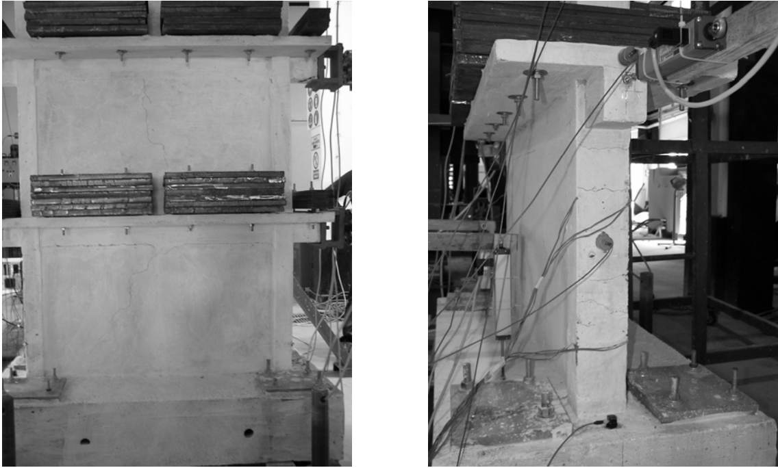
Figure 3.19. Diagonal cracks in the first and second story partition walls (left) and flexural cracks of the first story west column (right), at the end of first loading group
