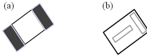
Figure 3.4 (a) Mask 1 for organic evaporation, (b) Mask 2 for metal evaporation.
