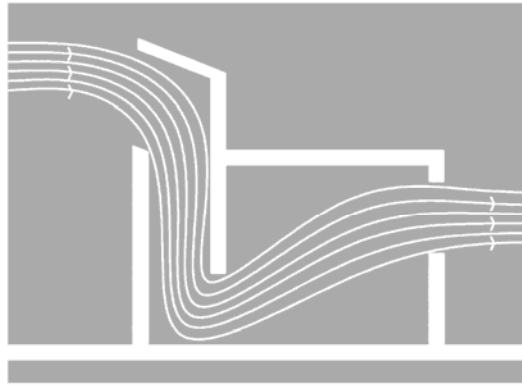
Figure 3.35: Schematic diagram of wind towers. Opening of the tower is facing wind direction.
