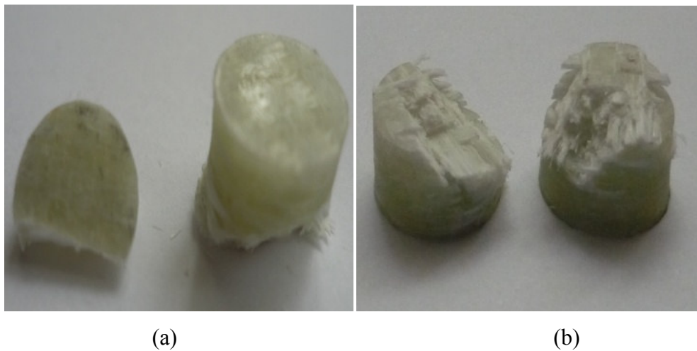
Figure 4.14. Photographs of samples tested in the through-thickness direction: (a) quasi-static and (b) high strain rate.
