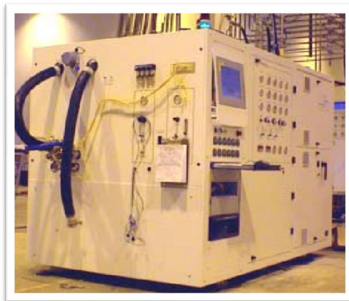
Figure 4.2. Up to 100 kW PEMFC power stack testing device (FCATS)
