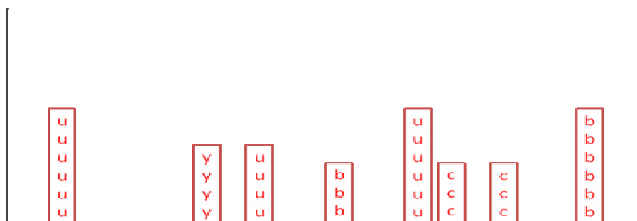
Figure 3.18. An Example of the Named Spectrum after applying the Running Sum and Peak Centering. The abundance of interesting peaks is increased and potential noise peaks are reduced.
