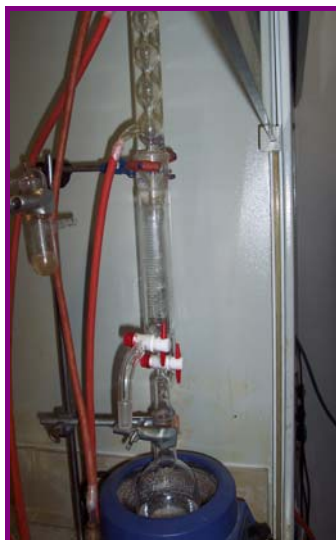
Figure 6.3. The experimental set up for drying methanol
