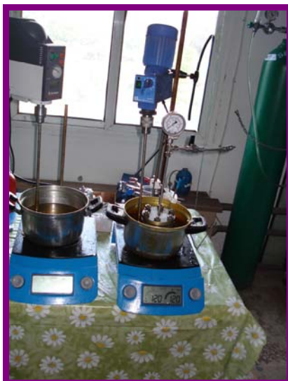
Figure 6.4. The experimental set up for rh-catalyzed carbonylative addition reactions of arylboroxines to alkynes
