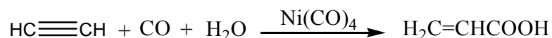
Figure 2.2. The synthesis of acrylic acid via nickel carbonyl catalyzed reaction in presence of CO and H 2 O (Source: Hancock 1973)
