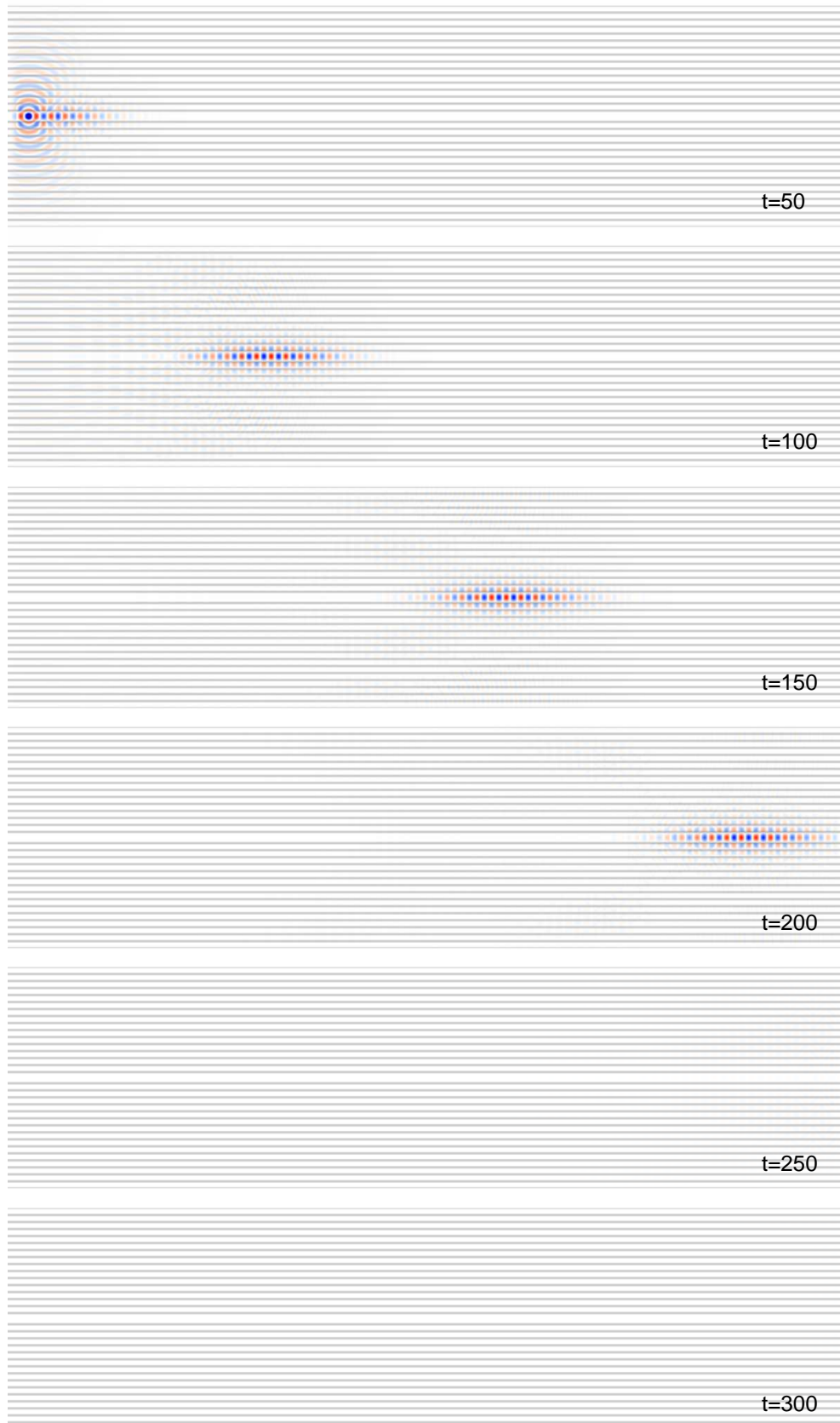
Figure 5.7. The z -component of the electric field, E_z(x, y) at different times for \omega = 0.60 \pm 0.1 . The group velocity is now non-zero, so the center of the gaussian wave packet moves at the group velocity, and expands very little in size because \omega(\beta) has very little curvature at this frequency.
