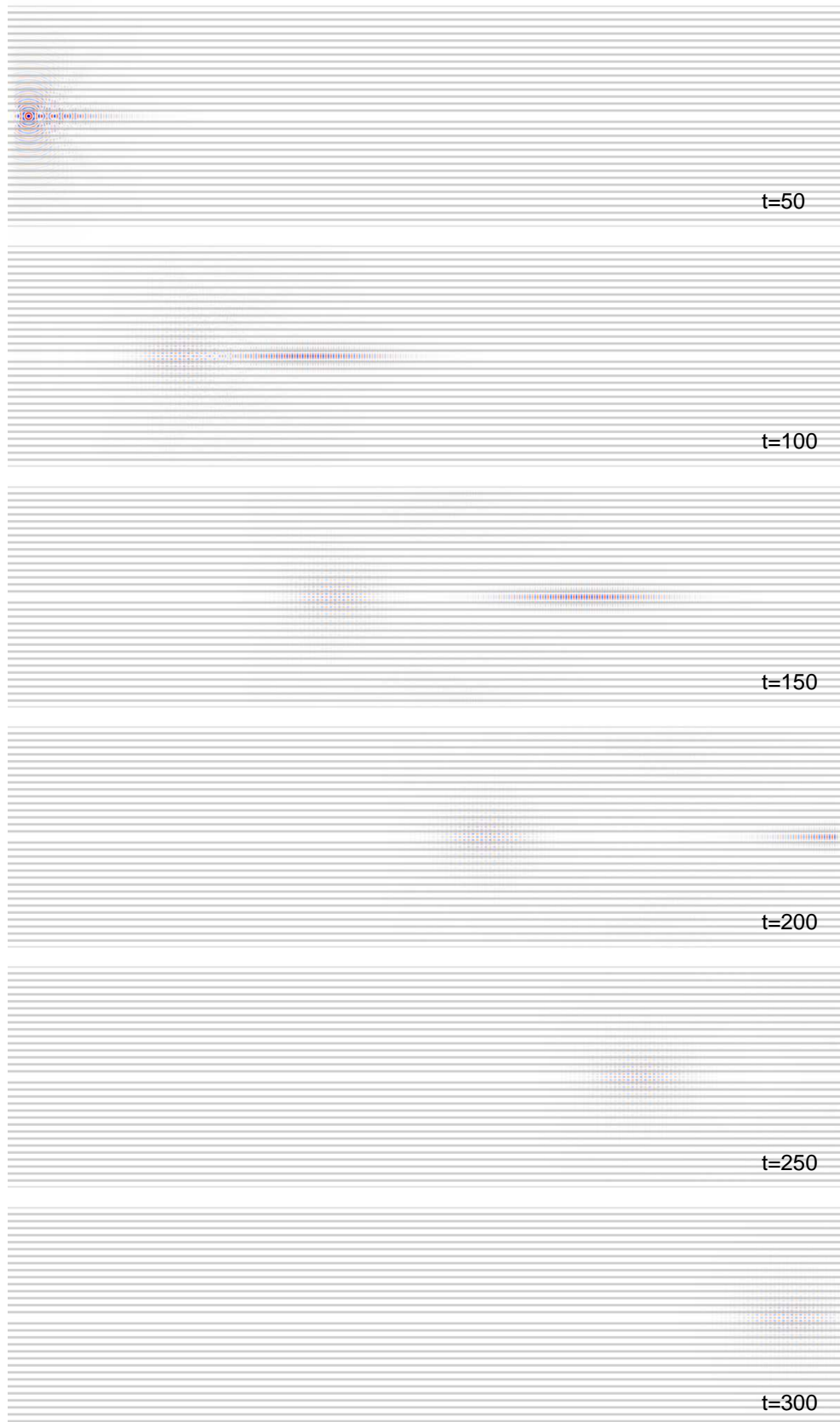
Figure 5.8. The z -component of the electric field, E_z(x, y) at different times for \omega = 1.40 \pm 0.1 . The waveguide is now multimode, with each mode moving at its own group velocity and spreading in size with its own dispersion.
