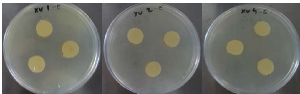
Figure 7.32. Growth inhibition of X. vesicatoria by zein film containing EUG (A: 1 mg/cm 2 ; B: 2 mg/cm 2 ; C: 4 mg/cm 2 )
