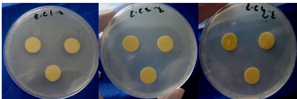
Figure 7.27. Growth inhibition of E. carotovora by zein film containing EUG (A: 1 mg/cm 2 ; B: 2 mg/cm 2 ; C: 4 mg/cm 2 )
