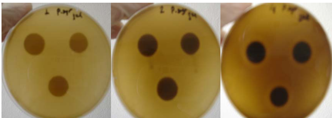
Figure 7.8. Growth inhibition of P. syringae by zein film containing GA (A: 1 mg/cm 2 ; B: 2 mg/cm 2 ; C: 4 mg/cm 2 )
