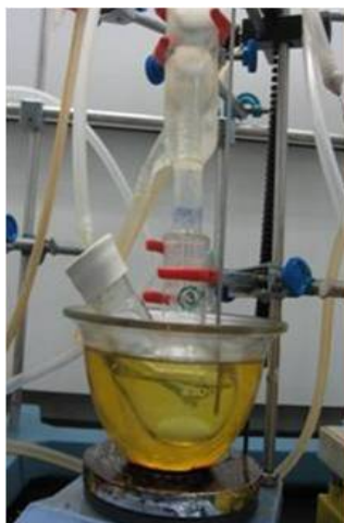
Figure 2.2. Photograph of experimental set up (two neck round bottom borosilicate reaction flask)
