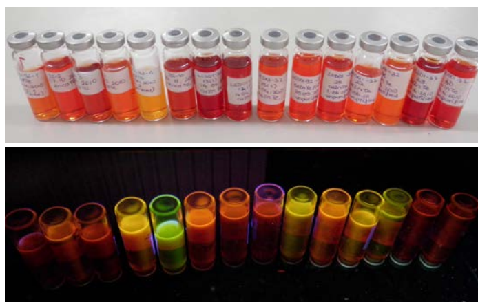
Figure 3.3. Images of Zn_xCd_{1-x}Te nanoalloys with different Cd:Zn ratio under day (above) and under UV light (below).
