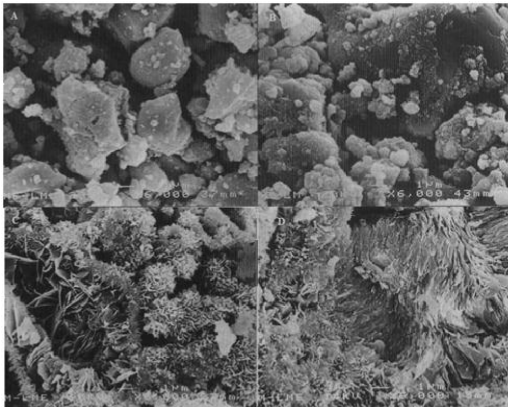
Figure 4.2. SEM pictures of cement at various periods of reaction: (a) after 15 min; (b) after 1 hr; (c) after 64 hrs; (d) after 360 hrs. (Source: Ginebra et al. 1997)
