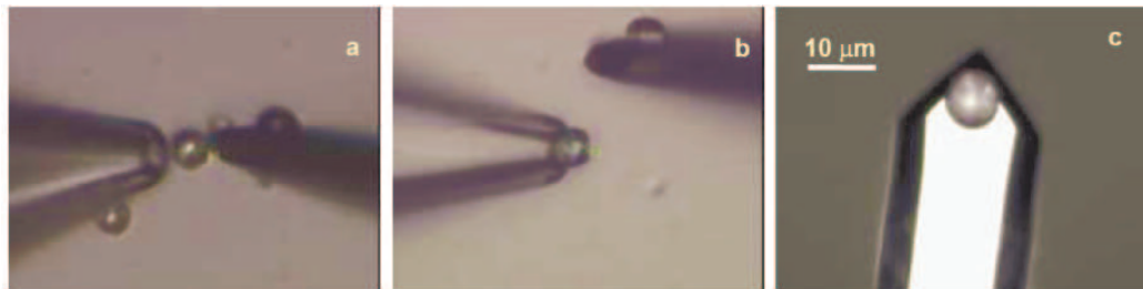
Figure 3.7. Manipulation of the colloid probes and placement on a triangular cantilever using micromanipulator system (the scale in 5-c applies to 5-a and 5-b also) (Source: Polat, et al. 2006).
