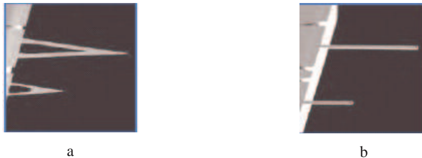
Figure 3.4. Types of cantilever used in AFM, a) Triangular cantilever, b) Rectangular cantilever (Source: Veeco Probe Catalog).
