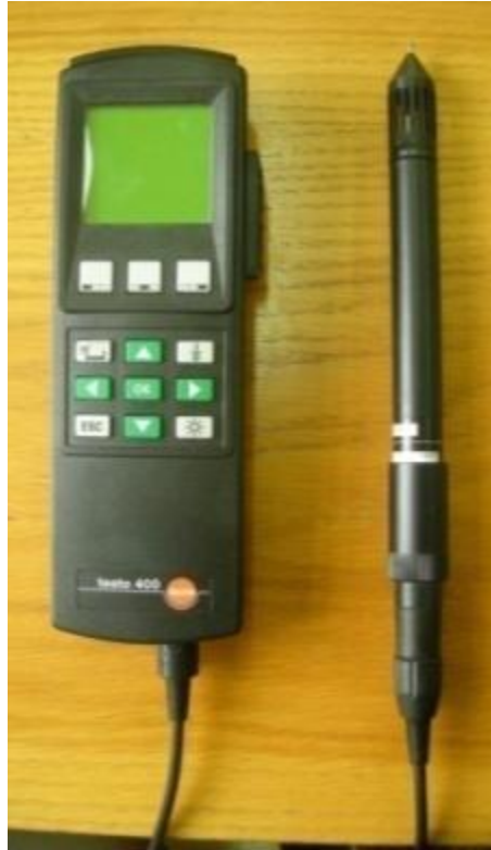
Figure 1.8. TESTO 400 *2 with 2 hot wire probes with measurement range 0m/s-10m/s wind speed for time limited measurements.
