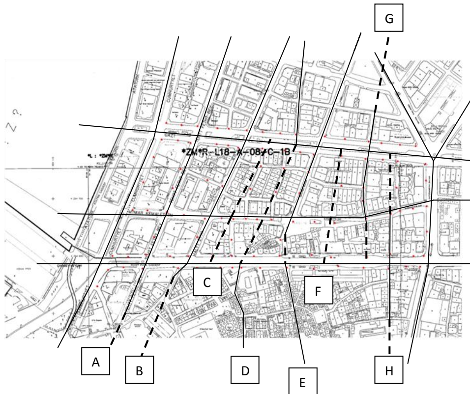
Figure 4.23. The Konak Site with the existing (____) and the potential air paths (___) on the planimetric (2D) level.
