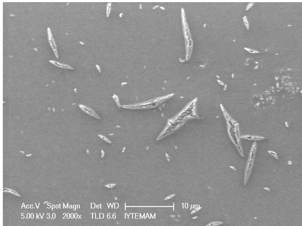
Figure 75. Alcoa alumina support (10% wheat starch, 1300° C / 2 hours), double wet coated (1.5 and 1 vol.% AKP-50 alumina, (3% PVA), 950° C / 2 hours), dip-coated via Zr colloidal sol (15 sec., 450° C / 2 hours).
