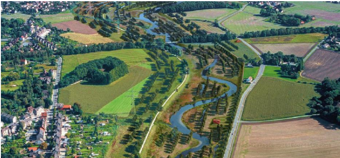
Figure 2.28. Natural channel design in Dortmund, Germany (Source: Prominski, Stokman, Zeller, Stimberg, & Voermanek, 2012)
