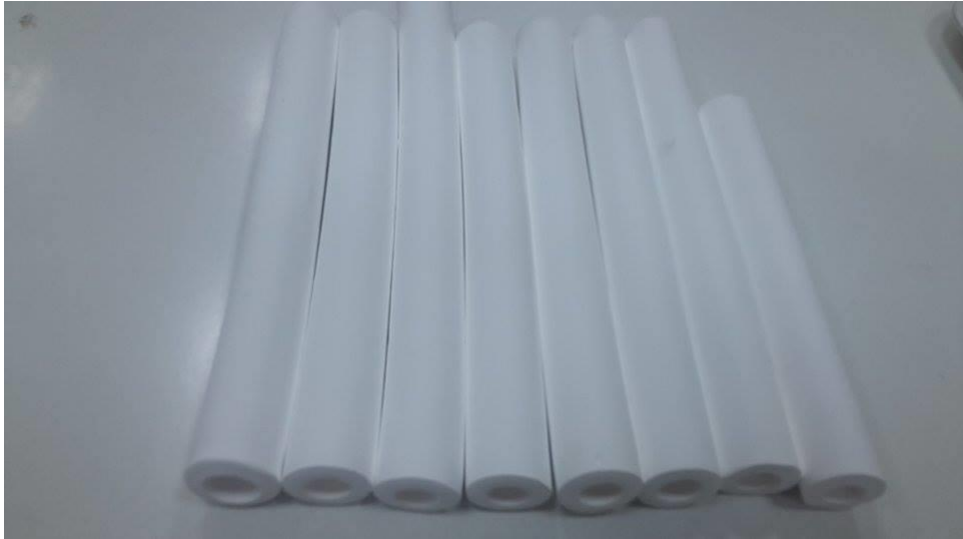
Figure 7.12. Extruded heat treated tubular alumina supports.
