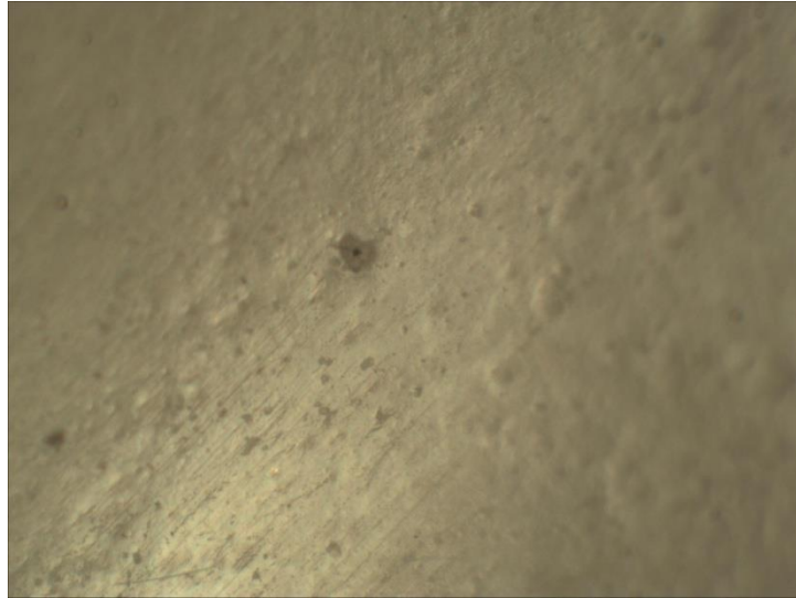
Figure 7.27. Optical microscope image of 0.5 \mu\text{m} \alpha -alumina coated membrane MF surface heated with 2°C/min rate to the peak 1200°C soak temperature.
