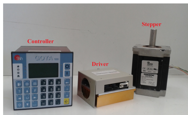
Figure 5.2. Control Setup Components
