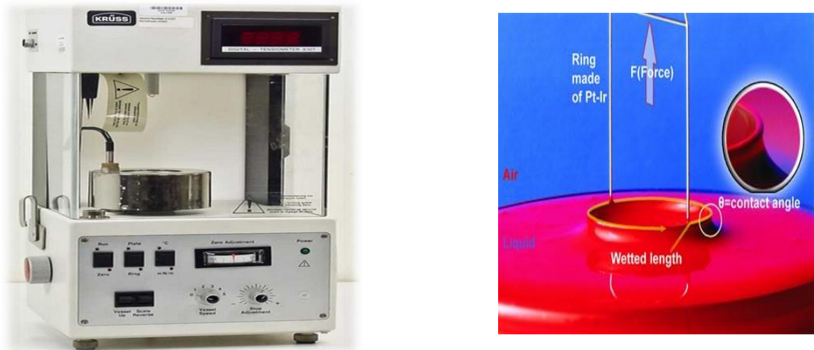
Figure 3.6. A Krüss model digital tensiometer (K10ST) used for surface tension measurements.
