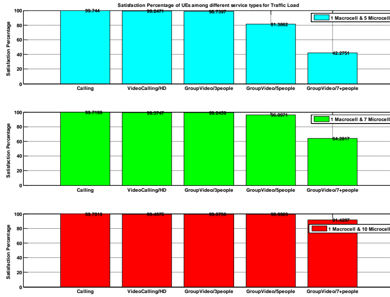
Figure 4.28. Satisfaction percentage for proposed traffic load based strategy with OFA Model 1 (Case 9.2, 9.3, 9.4)
