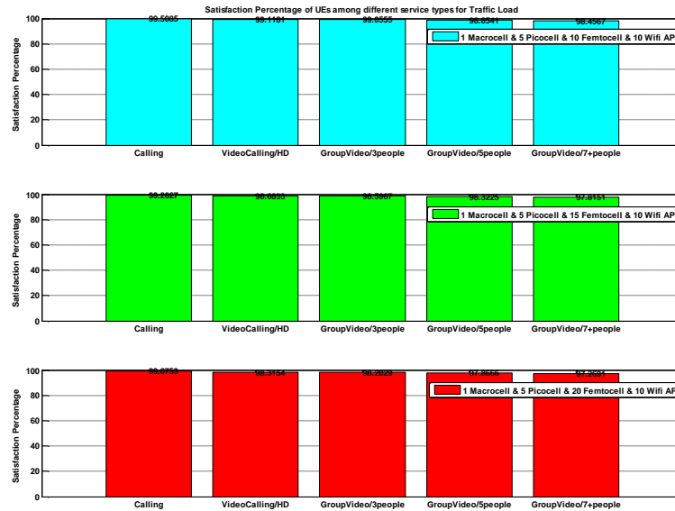
Figure 5.16. Satisfaction percentage for proposed traffic load based strategy with OFA Model 2 (Case 10.2, 10.3, 10.4)
